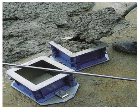
Fig. 2. Casting of Concrete Cubes (M50)
